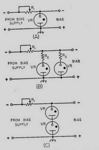
Fig. 12-29—Illustrating the use of VR tubes in stabilizing protective-bias supplies. R<sub>1</sub> is a resistor whose value is adjusted to limit the current through each VR tube to 5 ma. before amplifier excitation is applied. R and R<sub>2</sub> are current-equalizing resistors of 50 to 1000 ohms.
